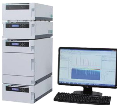
Figure 19- Column equipment GPC(Jasco, 2021)
